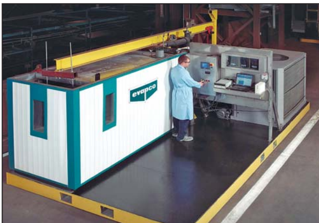
冰蓄冷系统试验台, 用于蓄冰设备制冰及融冰释冷时的性能评估 Thermal ice storage test unit with glycol chiller utilized for developing charge and discharge performance ratings
