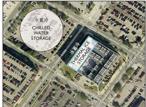
冰蓄冷比水蓄冷减少60%-80%的占地面积 Reduces thermal storage footprint 60%-80% less than stratified chilled water storage
