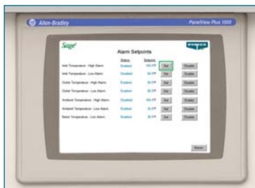
Alarm Setpoints Screen
